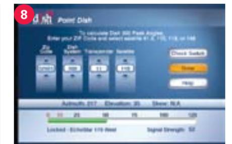
Satellite should be whatever satellite you want to point at. **The 72° satellite is recommended as a single satellite solution for DISH HD programming.** See “Compatible Satellites” for help.
