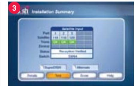
Make sure that there are no checkmarks by SuperDISH or Alternate. Select **Test**.
